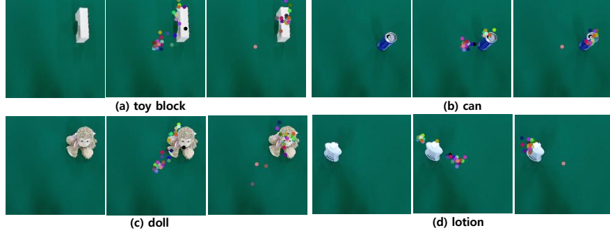
Fig. 4. Each left image of (a-b) is input image. Each center image of (a-d) displays values at feature points layer in Figure 2, in which DCNN^+ is pretrained using unsupervised learning. Each right image of (a-d) generated by pretraining DCNN^+ using the proposed supervised learning. Each feature is displayed in a different color.
